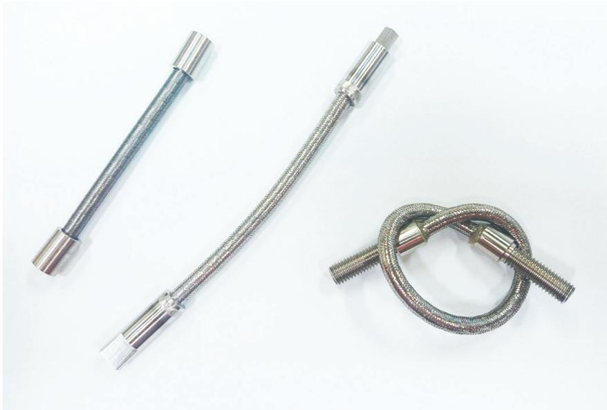
Fuji Beyond is a flexible tube comprising a single wound seamless wire that can be made from various alloys. Unlike Fujiloy, which is sintered and strong, Fuji Beyond is flexible and elastic, causing it to have characteristics of returning its original form after deformed by external forces.
